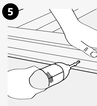
Pre-drill and countersink holes then fix, with one screw 100mm from each end and spaced no more than 500mm apart in between, checking units are straight and level
