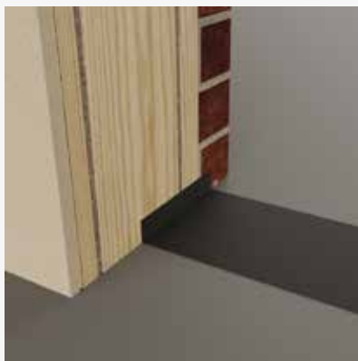
Line base of opening with DPC.
