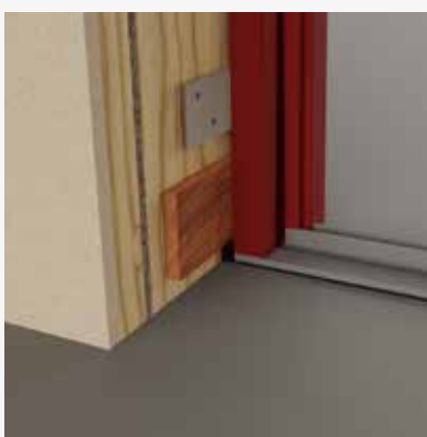
Wedge at the bottom of each side (opposing wedges from inside and outside) so the top can be adjusted without the bottom moving.
