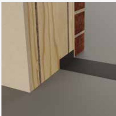
Line base of opening with DPC
