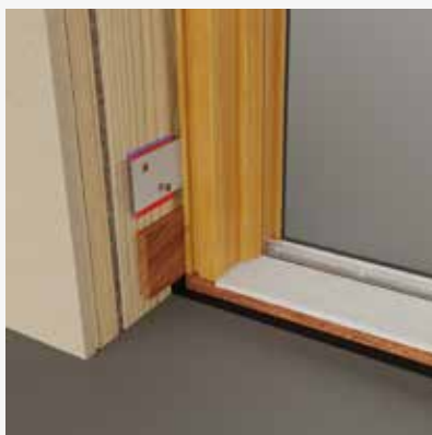
Nylon packers or steel shims must be installed on all four corners, behind the brackets. Once the product is level, square and plumb all fixings are added and tightened.
