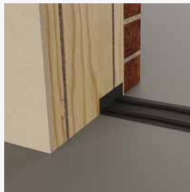
Apply two lines of mastic above & below DPC over the whole width
