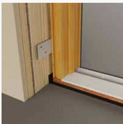
Place threshold onto a bed of mastic. Position frame in place according to a predetermined position.
